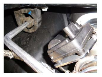
**Step 6.** If your vehicle has valves, re-connect the wiring harness plugs to the Valve motors and wire mounting bracket. If not yet purchased, Valve Kit is part# 10805
